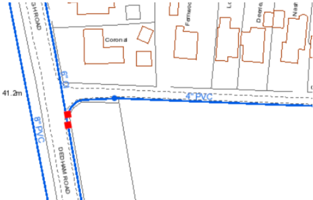
Figure 18: Potable water service.
